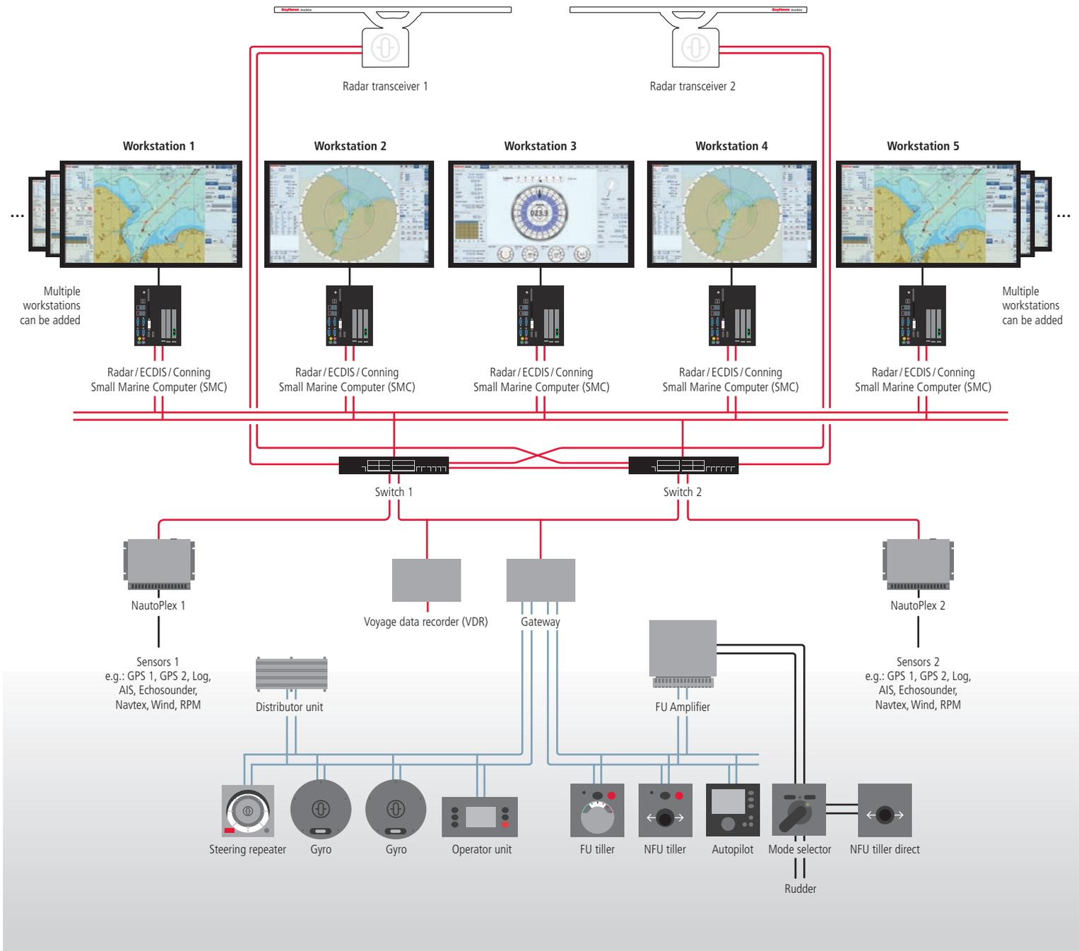
Synapsis NX fulfills basic IMO requirements as well as highest class notations such as NAUT (AW) and NAUT (OSV). The core components provide the backbone for the system and the shared services, workstations and applications can be flexibly added as needed in the individual project. The new system architecture reduces complexity of the system for easier installation, higher reliability and better resistance to failures.
