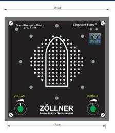
Einbauöffnung / cut out for Installation:  $138 \times 138$ mm Einbautiefe / plug-in depth: ca. / approx. 160mm IEC 60945, 4.4.b) protected from the weather
